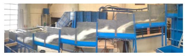
Figure 8. Hydraulic modelisation on the reoxygenation sill ( $Q = 50 \text{ m}^3/\text{s}$ )
